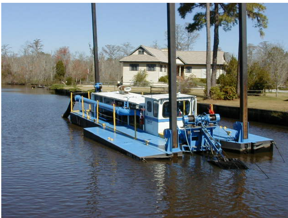
HYDRAULIC DREDGE OPERATING IN PLANTATION CANAL. DISCHARGE PIPE ENTERS WATER AT STERN OF DREDGE AND MOVES WATER AND DREDGED MATERIAL TO DIKED AREA SHOWN ON ACCOMPANYING PHOTO.
